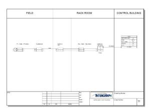
Loop drawing generated by SPI SmartLoop
